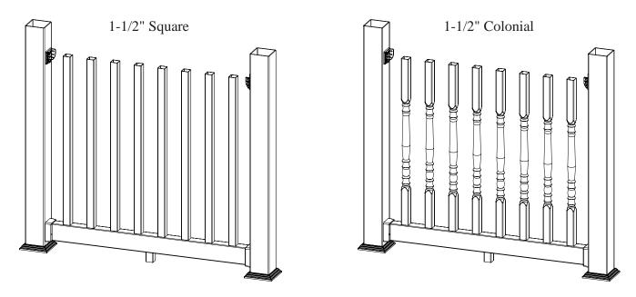
**Step 5 - Insert the balusters.** Having secured the bottom rail into place, insert the balusters into the bottom rail. If the 1-1/2" colonial balusters are being used make sure the balusters are inserted so the baluster tapers are uniformly installed.
