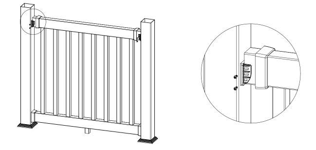
**Step 7 - Secure the top rail.** Position the top rail over the exposed ends of the balusters so that it is positioned on the resting flange of the installed nylon post brackets. Attach the top rail to the nylon post brackets by using the (4)  $\#10 \times 1"$  pan-head screws. Fasten two screws into each side of the nylon post bracket using the top and bottom slots of the nylon post brackets. Snap the 2" x 3-1/2" bracket covers positioned in Step 6 onto the nylon post brackets.
